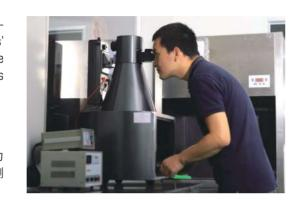
Multi-function lens test station: 透镜综合测试仪 Radius Focal length
