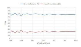
三通道滤光膜 Triple Bandpass Filter Coating
