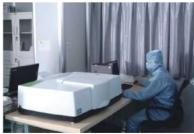
Lambda 750 spectrophotometer: 分光光度计 Transmittance Reflectance
